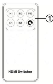
① IN1、IN2、IN3、IN4、IN5: Press this button will force switch the input port and the LED will indicate the corresponding input source. Note: IN4、IN5 in  $3 \times 1$  Switch product is no function.
